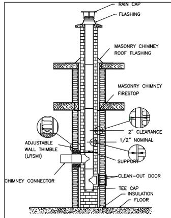
Fig. 4 - New masonry liner installation for interior chimney
